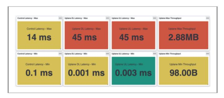
ASN Latency Measurement for control and User plane packets
